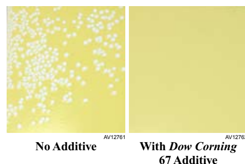
Figure A. Water-Reducible Stoving Paint – With and Without Dow Corning 67 Additive
