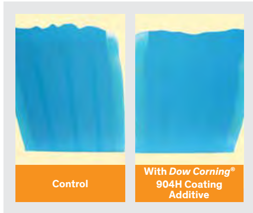
Figure 3. Improvement of water beading (WCA)
