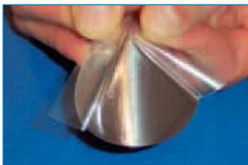
**Figure 2 – A transdermal drug delivery patch using a silicone pressure sensitive adhesive.**
