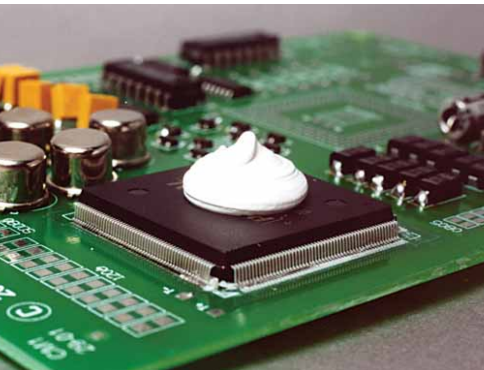
Thermal grease is one of the best performing TIMs. Photo courtesy Dow Corning Corp.
