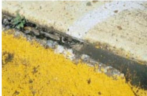
*Comparisons of test joints at Eglin Air Force Base indicate that while organic sealants have become brittle and the joints failed, the silicone sealants exhibit excellent adhesion and flexibility.*
