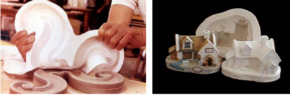
Figure 2. Flexible one-piece block molds: a silicone mold being separated from a PU copy (left); a silicone mold, and two copies, one after and one before finishing (right). Pictures courtesy of Dow Corning.
