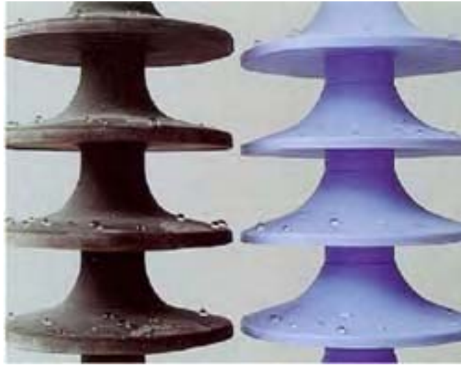
Figure 2. Comparison of an insulator after 23 years of use and exposure to pollution (left) vs. a retained sample kept at RT (right). Both still show excellent hydrophobicity as indicated by the high contact angle of the water droplets. (Picture courtesy of Lapp Insulators GmbH & Co.KG).
