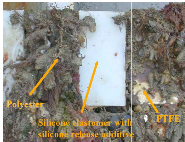
Figure 5. Extent of fouling of coating steel panels submerged for two-and-a-half years in the English Channel. Picture courtesy Dow Corning Ltd.
