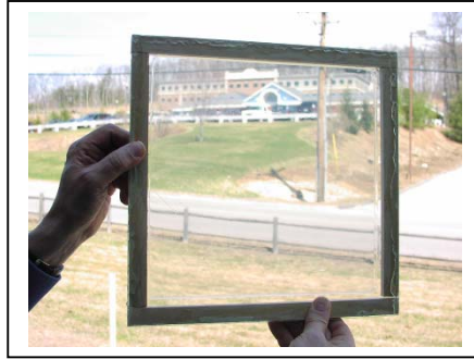
Figure 7 – Highly transparent aerogel interlayer system (Courtesy of Aspen Aerogels)
